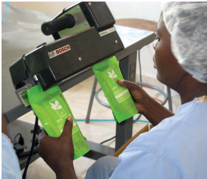
RELIABLE SEALS. The new band sealer provides consistent time, temperature and pressure, resulting in reliable seals for the RUTF product.
